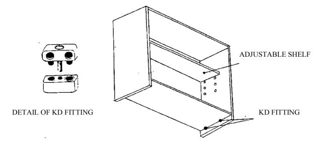
(a) The KD fitting is manufactured from a plastic material using the injection moulding process.
